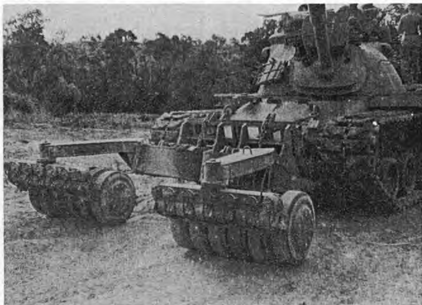
DEFENSIVE WEAPON—This machine, which searches out enemy road mines, is now in operation by Company E, 4th Engineer Battalion. The big wheels on the front detonate the mine causing damage only to that part of the vehicle. And these are easily replaced.
